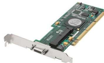
Targeta PCI-E per discs durs SAS (Serial Attached SCSI) (connectors 4 canals intern i 4 canals extern) (suport RAID 0,1,1+0)
