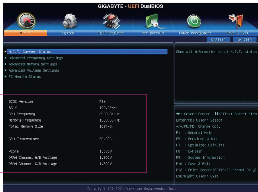
This section provides information on the BIOS version, CPU base clock, CPU frequency, memory frequency, total memory size, CPU temperature, Vcore, and memory voltage.
